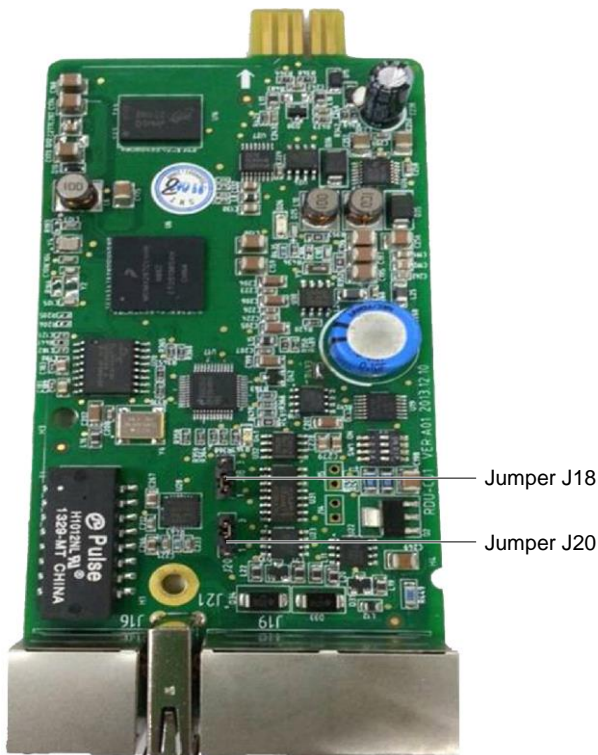
Figure 2-1 Jumper locations of the RDU-SIC G2 card
