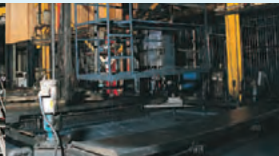
Autophoretic coating of frames — Assures complete coverage for maximum corrosion protection.
