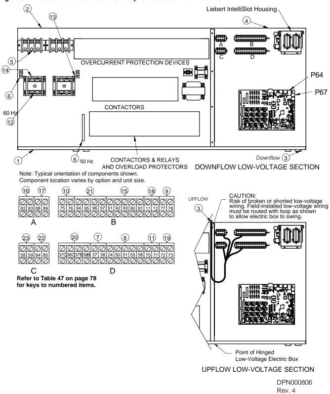
Figure 61 Electrical field connections for upflow and downflow models
