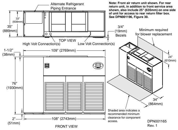
Figure 17 Cabinet and floor planning dimensions—upflow, air-cooled, 53-77kW (15-22 ton), semi-hermetic compressor models
