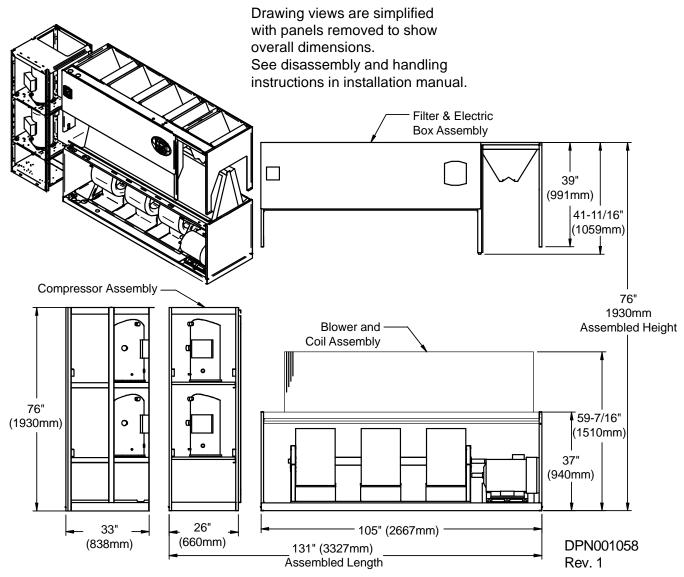
Figure 50 Component dimensions—downflow, air-cooled, 105kW (30 ton), scroll compressor models; forward-curved and EC fan
