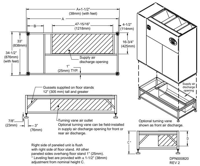
Figure 22 Floor stand dimensions—downflow, 28-42kW (8-12 ton) models
