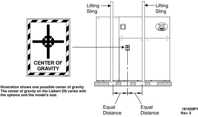
2. Place the slings between the bottom rails of the Liebert DS and the top of the skid.
