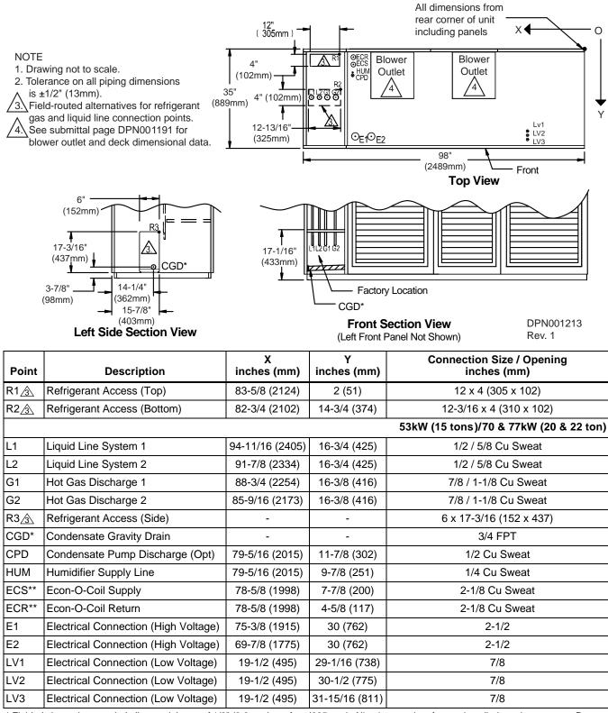
\* Field-pitch condensate drain line a minimum of 1/8" (3.2 mm) per foot (305 mm). All units contain a factory-installed condensate trap. Do not trap external to the unit. Drain line may contain boiling water. Select appropriate drain system materials. The drain line must comply with all local codes.
