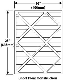
The filter pleat direction should run parallel to the direction of the short side of the filter , as shown above. Do NOT use long pleat filter construction , as shown at right above, because it can result in filter collapse.
