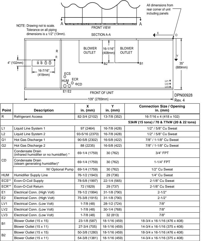
\* Field pitch condensate drain line a minimum of 1/8" (3.2 mm) per foot (305 mm). All units contain a factory-installed condensate trap. Do not trap external to the unit. Drain line may contain boiling water. Select appropriate drain system materials. The drain line must comply with all local codes.
