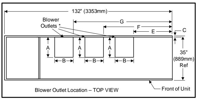
Figure 29 Blower outlet and deck dimensions—upflow 105kW (30ton)
