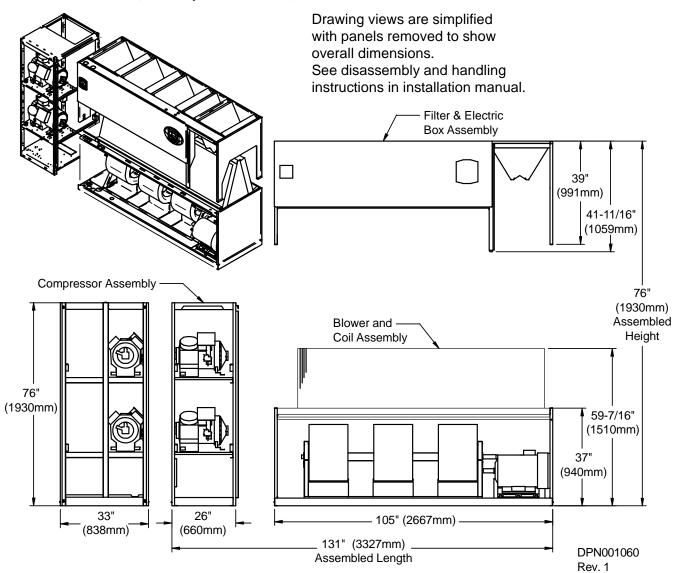
Figure 51 Component dimensions—downflow, water/glycol/GLYCOOL, 105kW (30 ton), forward-curved and EC fan, all compressor models; forward-curved and EC fan
