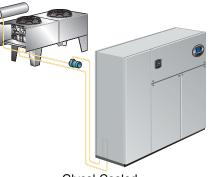
Glycol-Cooled Glycol-cooled units are factory-charged and tested. Field-installed piping is required from the unit to the drycooler and pump package.
