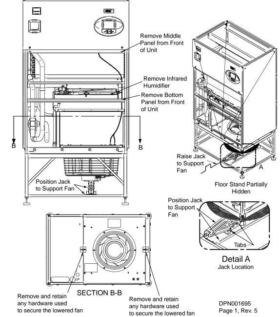
Figure 41 Removing the EC fans, Steps 1 through 5
