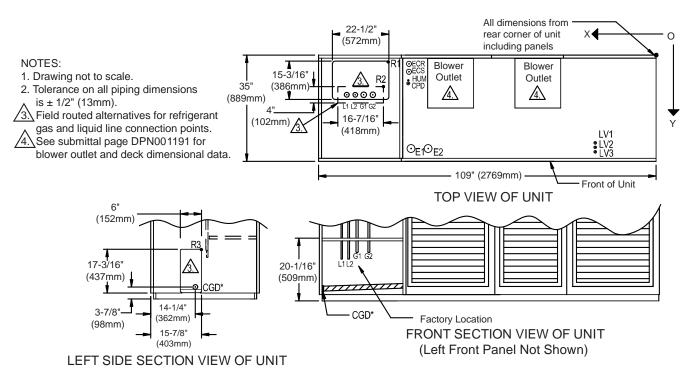
\* Field pitch Condensate Drain line a minimum of 1/8" (3.2 mm) per foot (305 mm). All units contain a factory installed condensate trap. Do not trap external to the unit. Drain line may contain boiling water. Select appropriate drain system materials. The drain line must comply with all local codes.
