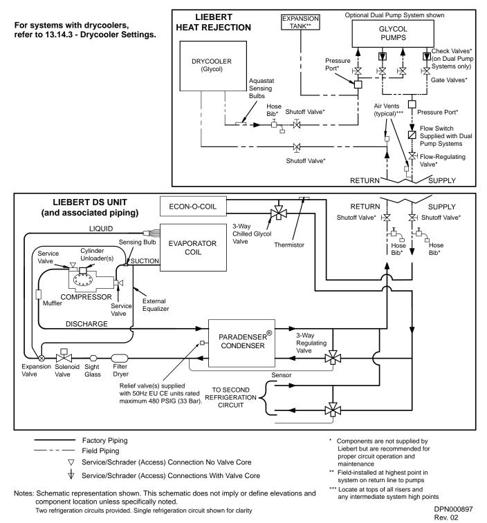
Figure 71 Piping schematic—GLYCOOL semi-hermetic compressor models
