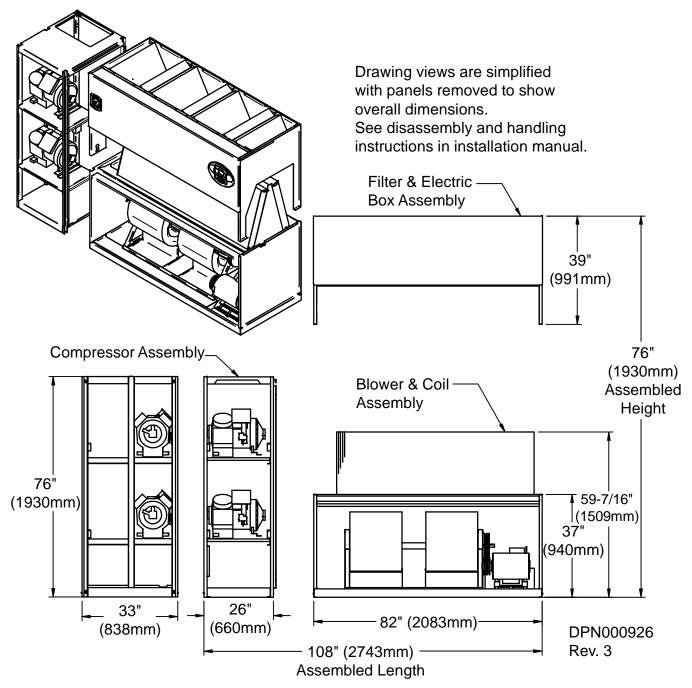
Figure 46 Component dimensions—downflow, air-cooled, 53-77kW (15-22 ton), semi-hermetic compressor models; forward-curved and EC fan
