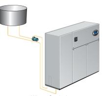
Water-Cooled Water-cooled units are factory-charged and tested. Field-installed water piping is required from the unit to the cooling tower.
