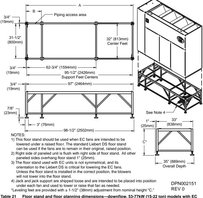
Figure 24 Floor stand and floor planning dimension, downflow 53-77kW (15-22 tons) models with EC fans
