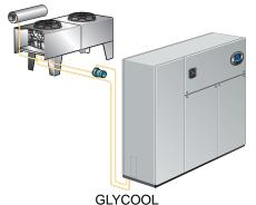
GLYCOOL units are factory-charged and tested. Field-installed piping is required from the unit to the drycooler and pump package. An additional coil is included for use when fluid temperatures are sufficiently low (below room temperature). Cooling is provided by circulating cold glycol through this second coil, reducing compressor operation.
