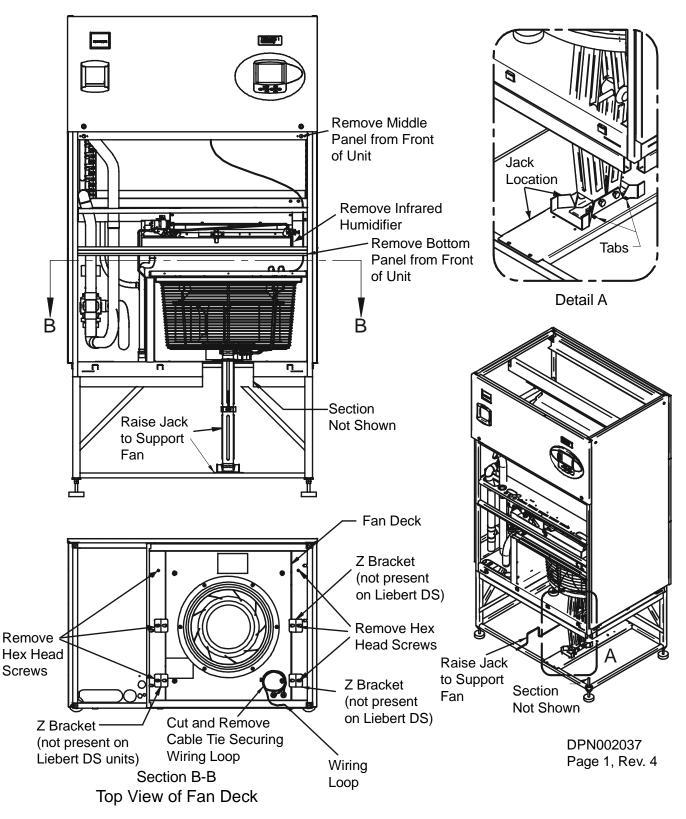
7. Using the jack, lower the fan module slowly until it rests on the frame of the unit.
