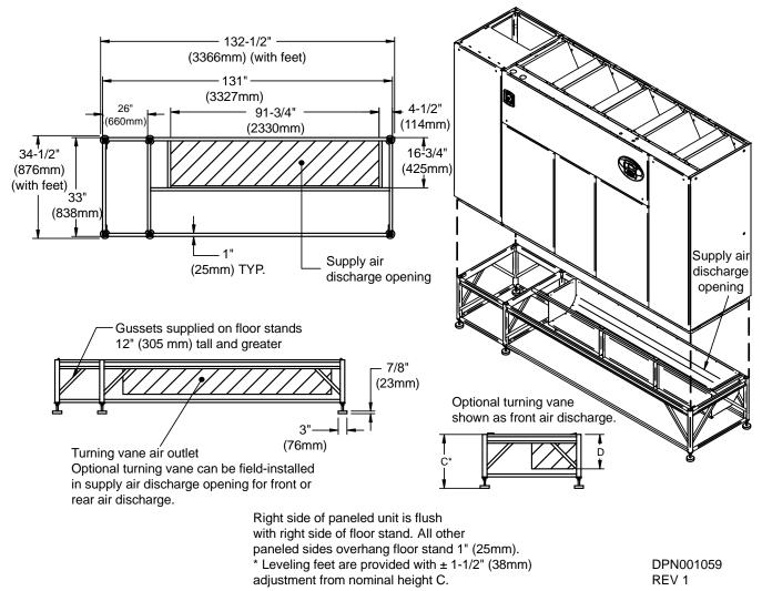
Figure 25 Floor stand dimensions—downflow, 105kW (30 ton) models
