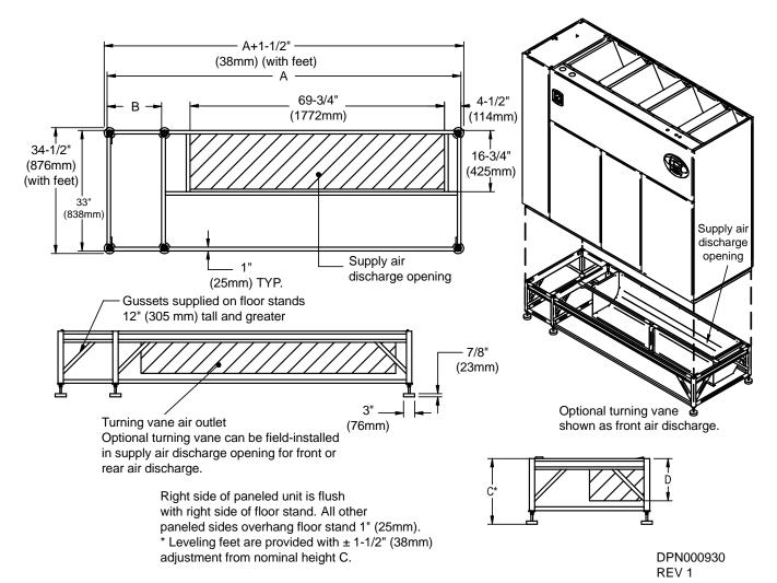
Figure 23 Floor stand dimensions—downflow, 53-77kW (15-22 ton) models
