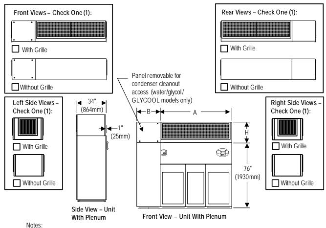
1. Typical 53-77kW (15-22 ton) unit orientation shown with grille plenum .
