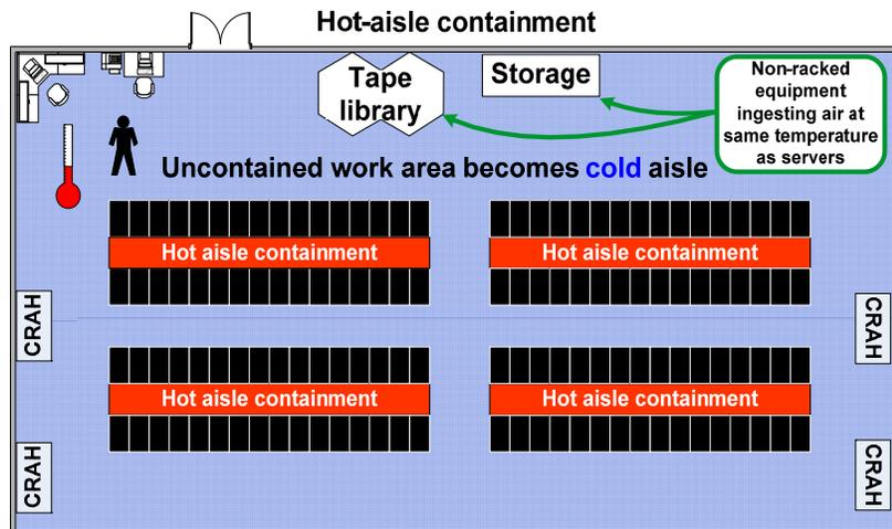
With CACS, high temperatures in the hot aisle cause the uncontained area to reach the same temperatures which can be problematic for IT personnel who are permanently stationed at a desk in the data center. With HACS, high temperatures in the hot aisle stay confined to the hot aisle and therefore do not affect IT personnel permanently stationed in the uncontained area.
