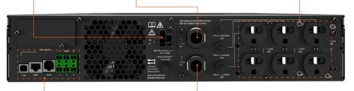
**Communications** SNMP, Serial, Dry contact, Local USB Local and remote configuration and UPS Management NEMA L5-30P input with over current protection Simple installation and power on with connected input cord
