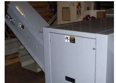
Covered Discharge Conveyor and bolted access panels
